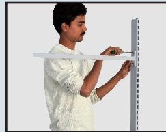
Fixing of Tie Bar on uprights
